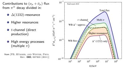
Especially "Multi  $\pi$ " contribution leads to change of flux shape; neutrino flux higher by up to a factor of 3 compared to WB treatment
