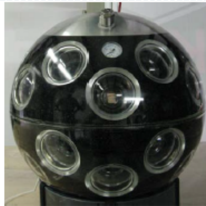
Multi-PMT Optical Module 31 small PMTs (3-inch) inside a 17 inch glass sphere
